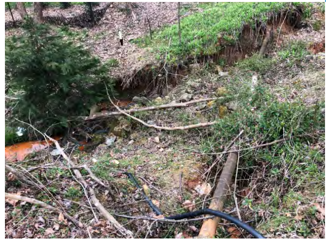
J. E. Broyhill Park (Lenoir, NC) gully monitoring equipment with the rain gauges and autosampler on the left and the groundwater well and sample tubing on the right. Note the exposed sewer line in the right photo.
