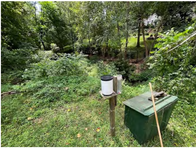
J. E. Broyhill Park (Lenoir, NC) gully monitoring equipment with the rain gauges and autosampler on the left and the groundwater well and sample tubing on the right. Note the exposed sewer line in the right photo.
