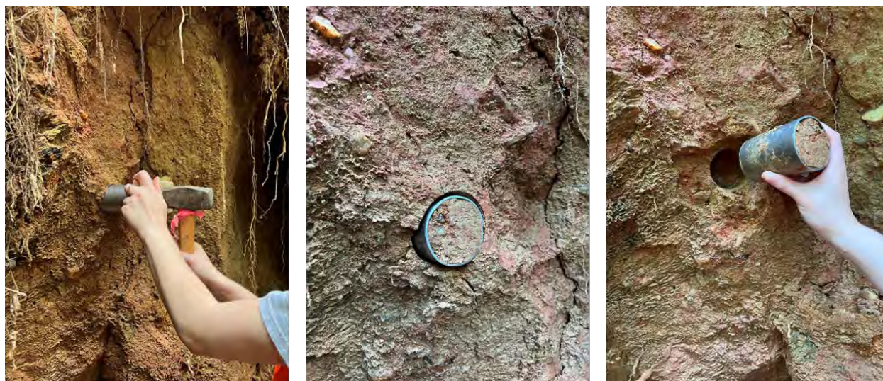
Figure 39. Collecting soil samples in the field.
