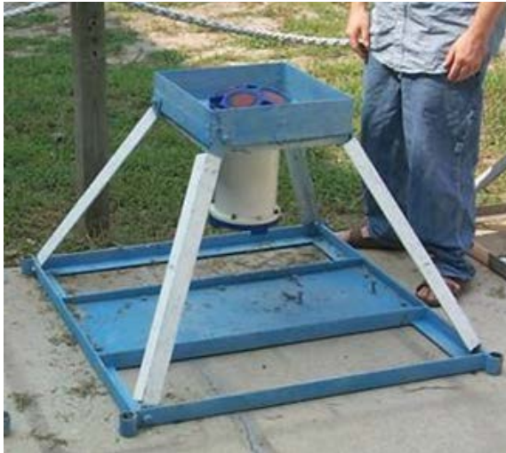
Figure 3. Acoustic Doppler Current Profiler (ADCP) in a typical mounting stand.
