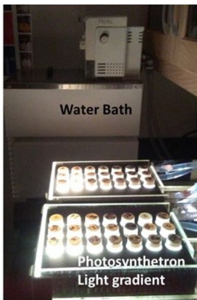
Figure 1. Photosynthetron set up for measuring the light vs. photosynthesis relationship. Note light increases from left to right within rows and also varies within columns.
